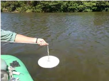
透明度測定状況<br>
